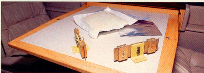
Three reasons for the C90B's quieter interior: dynamic vibration absorbers (foreground), bagged insulation (center), and thick foil swatches to defeat oil canning.
